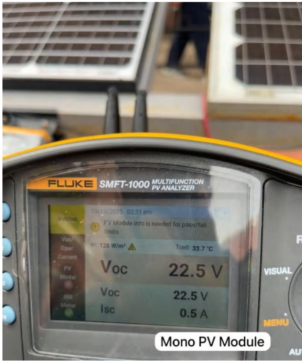
Fig. 3. Test result from SMFT-1000.
